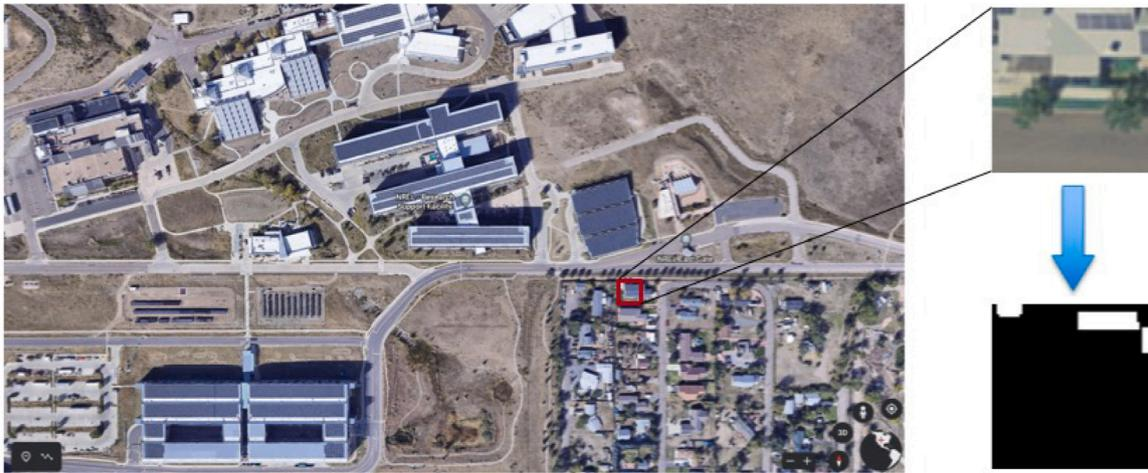
**Fig. 7.** A satellite aerial image-based PV detection procedure. PV panels are detected by well-trained machine/deep learning models in a small image patch that is extracted from a large image patch around the National Renewable Energy Laboratory campus. PV capacity can be derived from the detected images based on the pixel area and the roof tilt angle.
